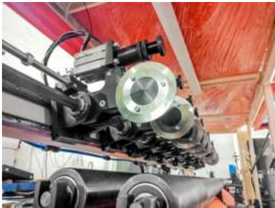
ZİNCİRLİ BİÇAK DÖNDÜRME SİSTEMİ / Knife turning system with chain
